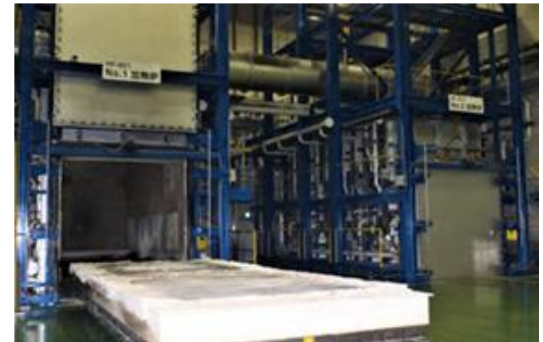
Battery recycling* (The furnaces to inactive batteries of ECO-SYSTEM AKITA CO., LTD)
